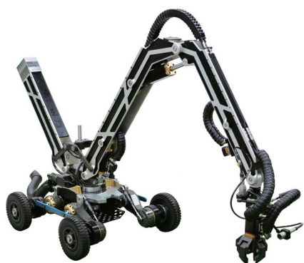
Gibbon (KNR's Hydraulic Mobile Robot in a nuclear power plant) (Body: 10^5 (Rad/hr), Grip: 10^6 (Rad/hr))
